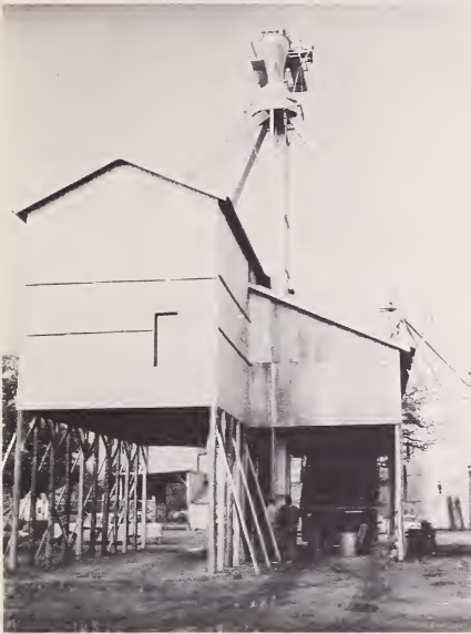
FIGURE 9.—Spout type automatic sampler for drawing inspection samples of farmers' stock peanuts as the peanuts are being conveyed from the unloading pit to holding or storage bins.
